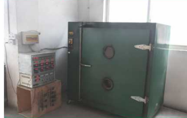
HIGH TEMPERATURE TEST CHAMBER
